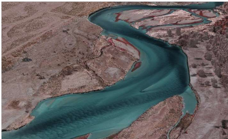
Topobathymetric lidar bare earth model with point cloud overlay colored by NIR imagery, Platte River, NE.
